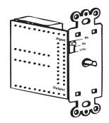
To prevent from overloading and damaging the amplifier, the switch must be set correctly to match the impedance of the speaker system to a level equal to or greater than the impedance of the amplifier.
